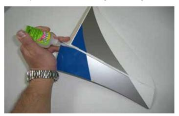
$\Box$  step 4 Check the alignment of the rudder and fuselage, than glue the rudder with some drops of medium CA, as per pictures.
