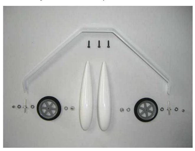
$\square\square$  step 2 Install wheel and wheel pant as per pictures.
