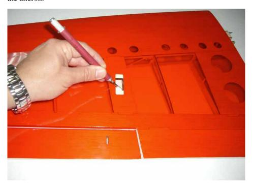
$\square\square$  step 3 Install the servo hardware (gommets and eyelets) and put the servo into the wing panel, as per pictures.
