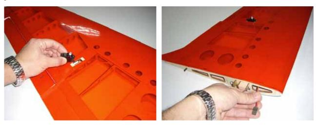
□□ **step 4**Drill using a 1,5mm drill bit, and install the servo into the wing panel using a Phillips screwdriver.
