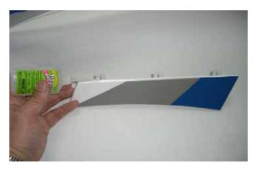
$\Box$  step 3 Carefully locate the rudder and glue the hinges with some drops of thin CA.
