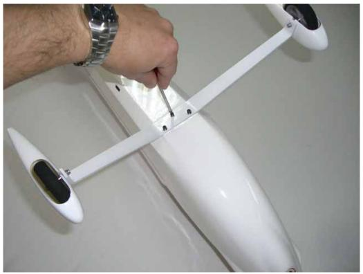
□□ **step 5**Test fit the L.G. Lift Generator and his alignment with the fuselage.
