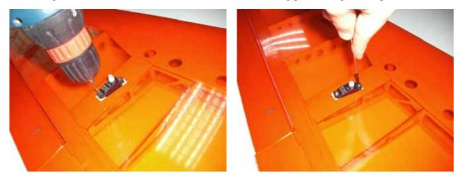
$\Box\Box$  **step 5** Glue the fibreglass horn with medium CA into the aileron.
