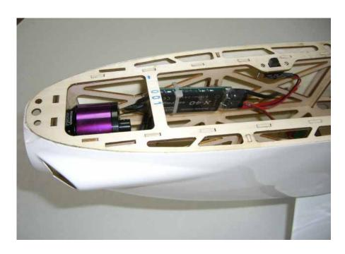
$\Box$  step 3 Glue with some drops of medium CA the Velcro strip included in the hardware pack.
