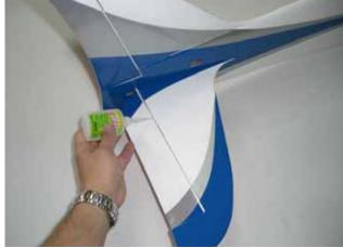
$\Box$  step 5 Once satisfied with the alignment, glue carefully with thin CA the stabilizer at the fuselage.
