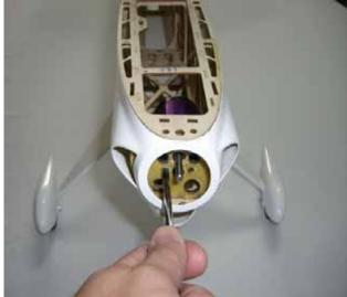
$\square$  step 2 Locate and fix the ESC and his switch as per picture.
