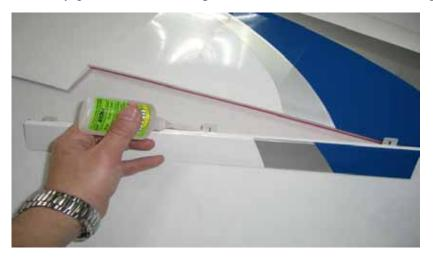
□□ **step 3** Locate the aileron and carefully glue, with some drops of thin CA, the hinges into the wing panel.
