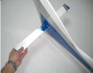
$\square$  step 3 Insert carefully the stabiliser into fuselage space and check the alignment with the rudder.
