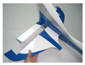
$\Box$  step 4 Locate the elevator hinges into the stabiliser. Glue carefully the hinges in the stabiliser with some drops of thin CA.
