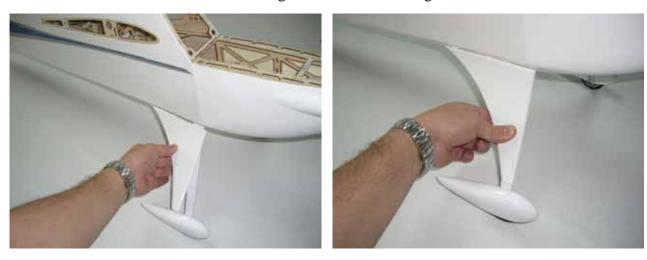
$\Box\Box$  step 6 Glue carefully the landing gear fillet with some drops of medium CA, as per picture.
