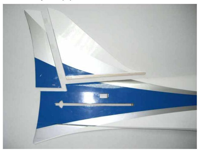
$\square$  step 2 Insert the three hinges in their appropriate slots of the rudder, and glue them with some drops of thin CA.
