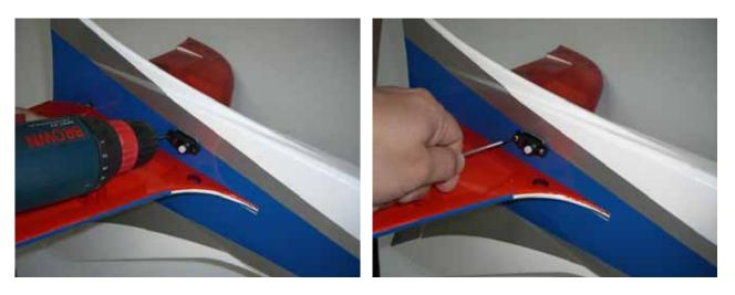
$\Box$  step 4 Glue the fibreglass horn with medium CA into the elevator. Than install the hardware and make the final adjustment as per picture.
