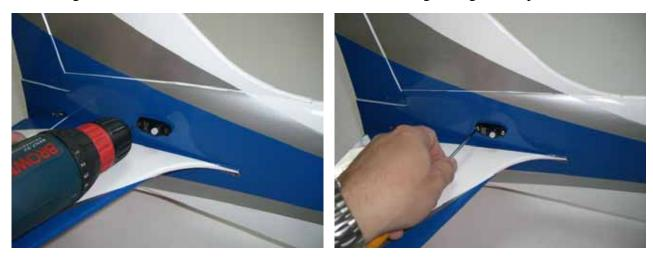
$\square$  step 4 Glue the fibreglass horn with medium CA into the elevator.
