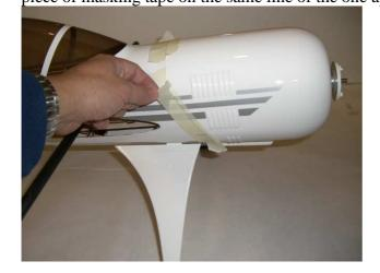
step 3Drill the location for the four self-tapping screws using a 1.5mm drill bit.Attach the cowl using the four self-tapping screws, included in hardware pack, and a Phillips screwdriver.
