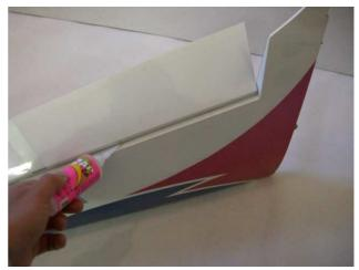
step 4Work the aileron up and down some times to work the hinges and check for proper movement.
