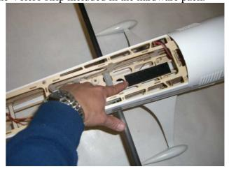
**step 2** Install the receiver, two extension 100mm for aileron servos and the battery pack as per the picture.
