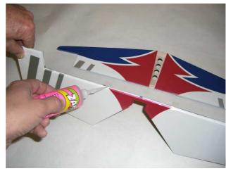
step 2Insert carefully the elevator through the fuselage.
