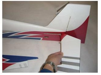
step 3Insert carefully the stabiliser into fuselage space. Locate the elevator hinges into the stabiliser.
