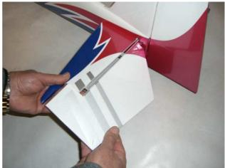
**step 4**Carefully glue the hinges in the stabilise with some drops of thin CA.
