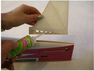
step 2 Insert the three hinges in their appropriate slots in the rudder. Verify the correct position-alignment and glue them with some drops of thin CA.
