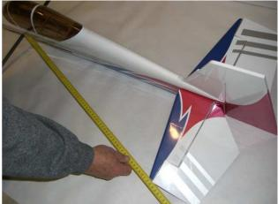
step 6Once satisfied with the alignment, glue with some drops of thin CA the stabilizer at the fuselage.
