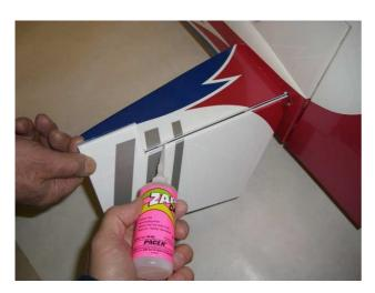
**step 5**Locate the carbon tube in his position and carefully check the alignment of the stabilizer with the fuselage.
