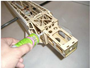
step 2Cut the two plastic air-scoops. Locate them on the mount and glue with thin CA, as per picture.
