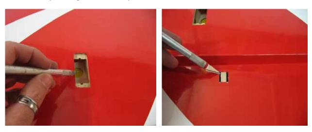
$\square\square$  step 3 Place the fibreglass control horn into aileron, check for correct alignment and glue it with some drops of medium CA.
