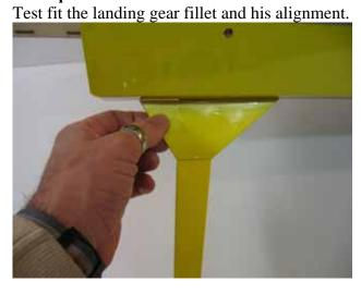
□□ **step 7**Once satisfied with the fit, glue the fillet on the landing gear using medium CA. Use the glue carefully avoid over runs on other areas.
