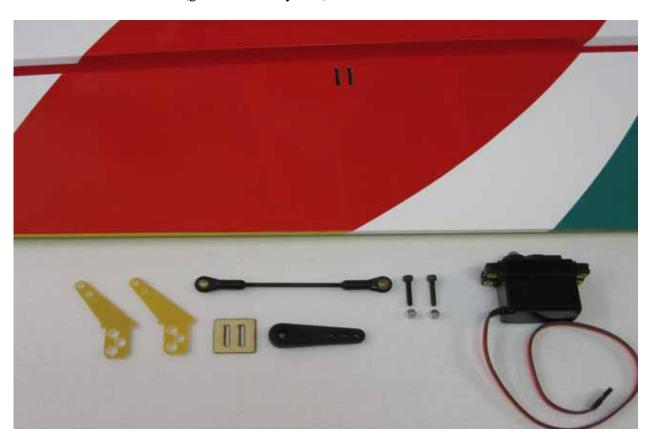
□□ **step 2** With the hobby knife open the servo bay and the control horn location.
