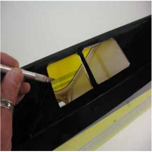
$\square$  step 5 Apply a piece of masking tape on the line were you have to make the holes for the cowl fixing screws, and mark the position as per the picture.
