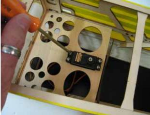
□□ **step 3** With the hobby knife remove the cover in the control horn location.
