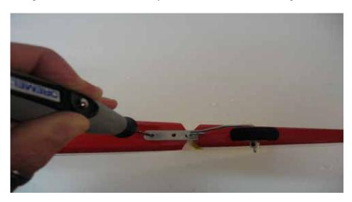
$\Box$  step 10 Use the two self-tapping screws to fix the tail wheel as follow.
