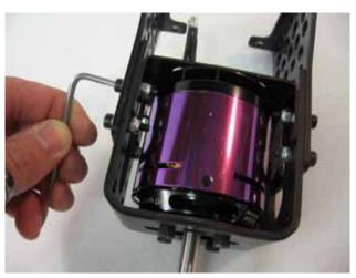
$\Box$  step 3 Drill the location of the blind nuts where it is marked on the firewall and install the 4 mm blind nuts included in the hardware pack. Check the right length of the mount and install it on the fuselage as follow.
