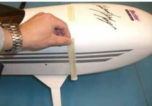
$\square$  step 7 Drill the location for the four self-tapping screws using a 1.5mm drill bit. Attach the cowl using the four self-tapping screws, included in hardware pack, and a Phillips screwdriver.
