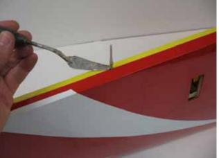
□□ **step 3** Carefully glue, with 5 minutes epoxy, the hinges into the aileron.
